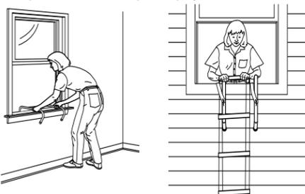
4. Exit carefully through the window and place your feet on the first rung. Hold onto the window frame until your weight is evenly distributed on the ladder. Climb down, keeping your body close to the ladder.
