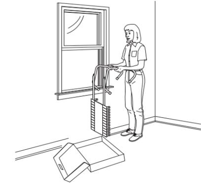
3. Place the sill hooks firmly over the windowsill and pull the release strap to deploy the ladder.
