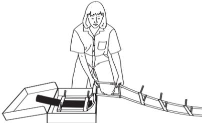
3. Use the plastic strap (attached to the last rung) to wrap and secure the rungs. This will minimize the chance of the ladder becoming tangled when you remove it from the box in an emergency.
