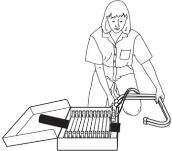
4. Place the folded sill hooks on top of the rungs, between the standoffs as shown in the diagram.
